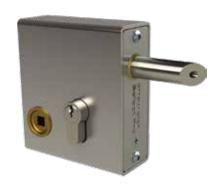
The weld-in latch deadlock has a latch and deadlock on the single bolt. The handles operate the latch and the key can then be turned to extend the deadbolt  $1\,3/16$ " (30mm) into the gate post to secure the gate.
