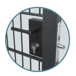
This bolt-on latch deadlock has both the convenience of a latch and the security of a deadlock. For day-to-day use, the handles operate the latch and this latch can then be deadlocked by turning the key.
