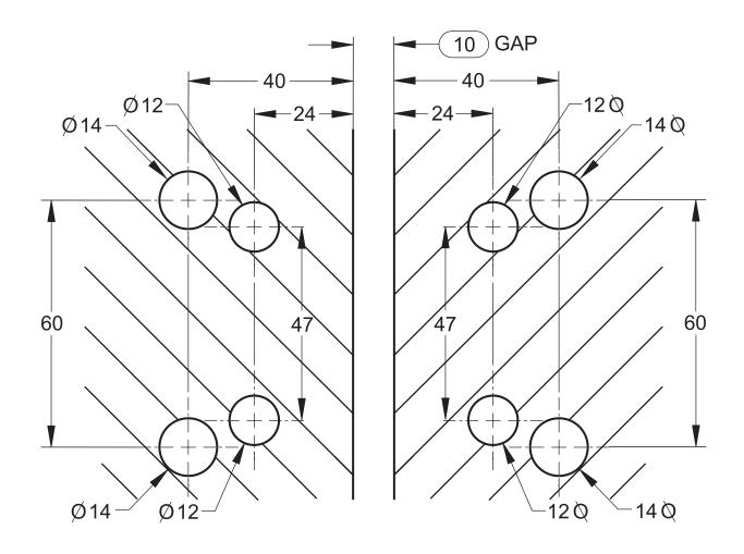
**GLASS CUT-OUT TOP AND BOTTOM** (ALL DIMENSIONS IN MILLIMETERS)
