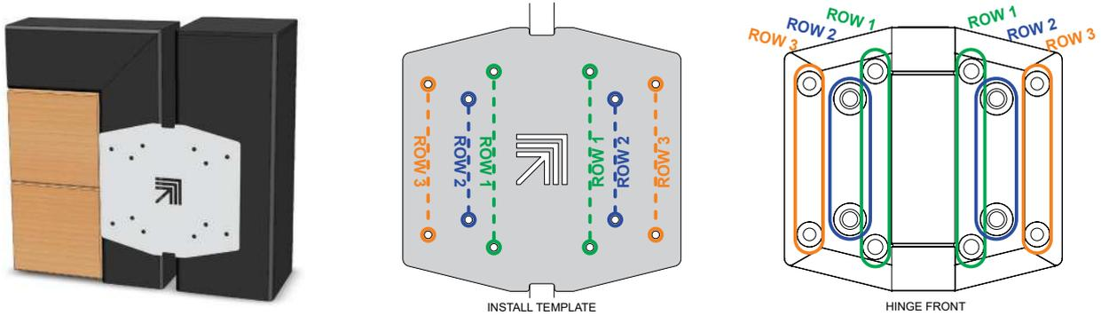
The unused fastener holes in the installation/hinge are for either re-alignment (**ROW 1 or 3** depending) after the first test IF there is a misalignment, and **ROW 2** which is for final securing of the hinges.
