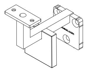
Back plate with 3 holes concealed by snap-fit plate cover. "Design Patent Pending"
