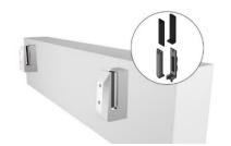
Install the L-Gasket, followed by the I-Gasket. Set up glass.
