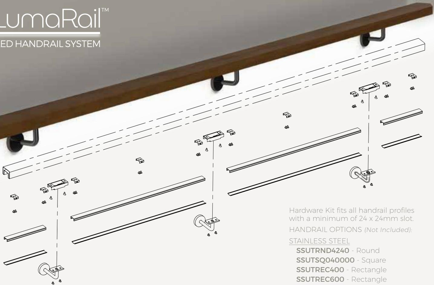
Hardware Kit fits all handrail profiles with a minimum of 24 x 24mm slot.
